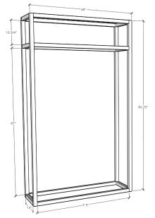
CUT LIST: 4 @ 82.25" 6 @ 45" 6 @ 13" PLY: 2 @ 48" x 16" Both of the large shelves are 48" wide and I used pocket holes to connect the frame pieces together. This allowed me to connect the 45" and 13" pieces on the same vertical plane.
